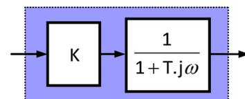
Gain en dB :  $G_{dB} = 20 \log_{10} |H(j\omega)| = 20 \log K - 20 \log \sqrt{1 + T^2 \cdot \omega^2}$
